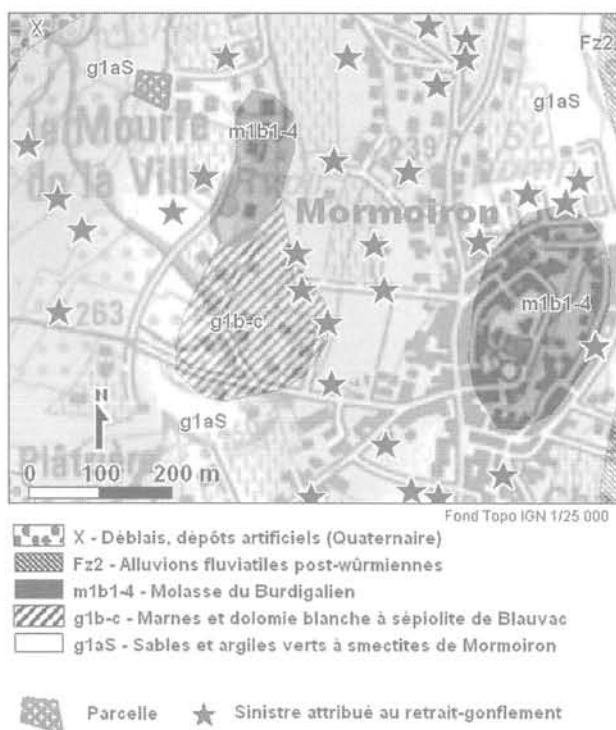
FIG. 3 Plan de situation de l'installation de Mormoiron (géologie extraite de la carte BRGM 1/50 000, feuille de Carpentras). Sketch map of experimental site in Mormoiron (from geological map of Carpentras at 1: 50,000, edited by BRGM).
